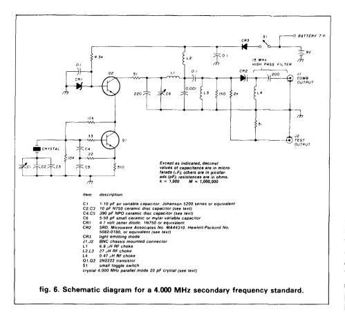
quite linear and can be decreased over a small temperature range (perhaps 10 to 40 degrees Centigrade) by simply placing a temperature compensating capacitor in series or parallel with the crystal.<sup>3</sup>
